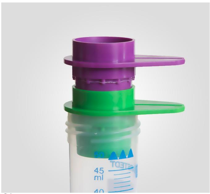
Stack  $Stacking \ of \ pluriStrainer @\ with \ different \ mesh \ sizes \ allows \ for \ straining \ various \ cell \ sizes \ at \ the \ same \ time.$
