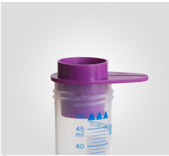
Filter Attach pluriStrainer® to a sterile 50 mL centrifuge tube. Then, add sample material onto the strainer and filter sample
